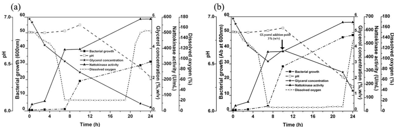
Figure 2. Changes in bacterial growth at 600 nm, glycerol concentration, natto kinase activity, pH and dissolved oxygen during the time course of fermentation for batch (a) and fed-batch (b) optimized conditions at 600 rpm, 2 vvm at 40 °C.
