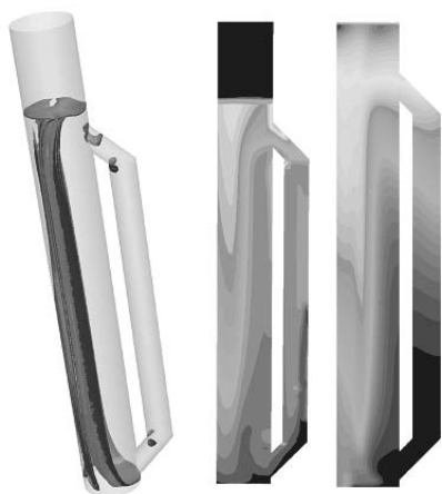
Figure 6. An airlift reactor has sparged air in the larger (riser) section and circulation through the narrower downcomer. The air-water interface (left), bubble size distribution (middle) and oxygen concentration (right) are shown.
